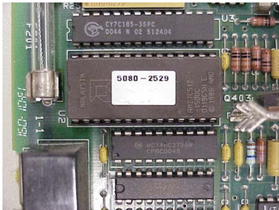
FIGURE 1 Tested PCA P/N 66103-61022 (Location of Circuit Reference “U2”)
